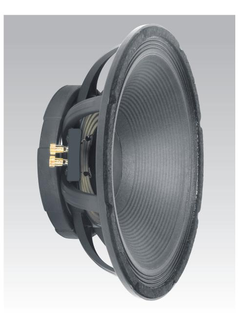
The magnet structure features a patented peavey technology: a one piece die-cast back plate/pole piece assembly. This construction eliminated an undesirable "air gap" in the magnet circuit, enhancing efficiency and reliability.
