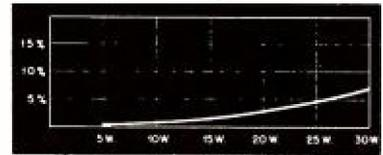
Fig. 3. Intermodulation distortion vs. power output.
