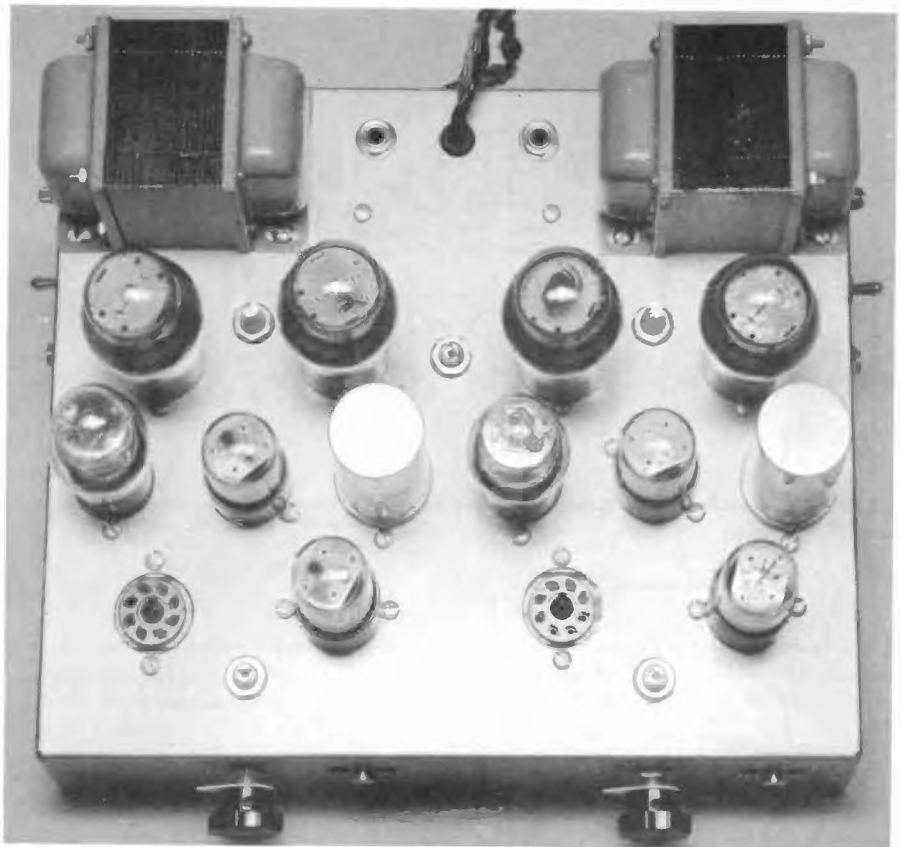
Fig. 4. Top view of the amplifier chassis. The jacks at the rear are for the outputs, while power is fed to preamps from octal sockets toward the front.
