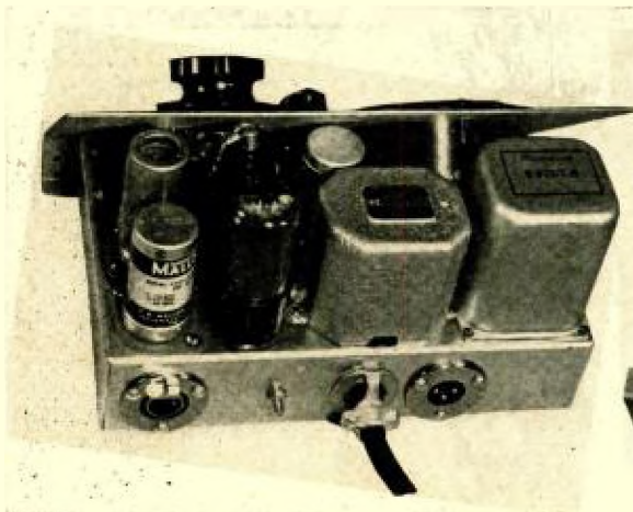
Fig. 8 (left). Top view of amplifier chassis, to show placement of major components. Fig. 9 (right). Under-chassis view of the amplifier.
