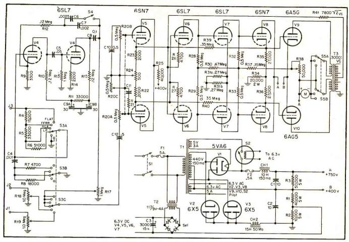
Fig. 2. Over-all schematic of the direct-coupled amplifier.
