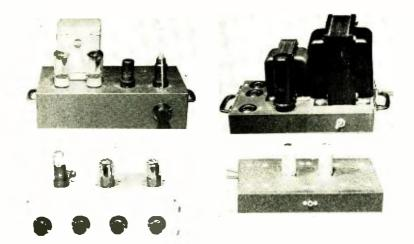
Fig. 5. Above, the preamplifier; below, the power amplifier. "Building block" construction makes for flexibility.
