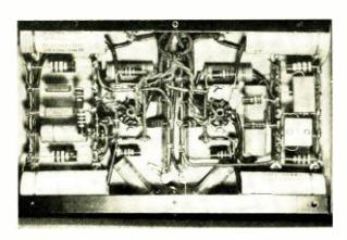
Fig. 9. Underside of dividing network chassis.
