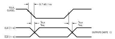
Figure 3. Propagation Delay, TCLK, CLKSEL to Outputs
