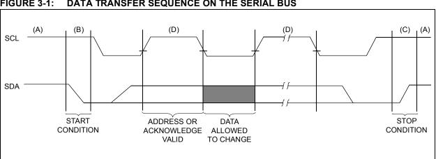
FIGURE 3-1: DATA TRANSFER SEQUENCE ON THE SERIAL BUS
