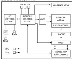
blocks. Functional address lines allow the connection of up to eight 24LC65's on the same bus for up to 512K bits contiguous EEPROM memory. Advanced CMOS technology makes this device ideal for low-power nonvolatile code and data applications. The 24LC65 is available in the standard 8-pin plastic DIP and 8-pin surface mount SOIC package.
