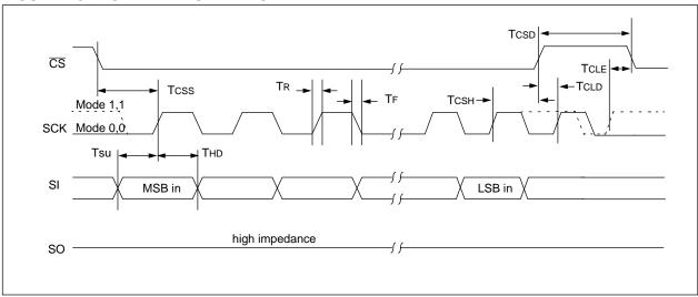
FIGURE 1-4: SERIAL OUTPUT TIMING
