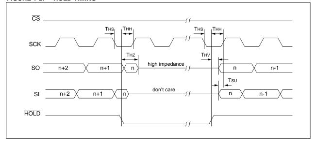
FIGURE 1-3: SERIAL INPUT TIMING
