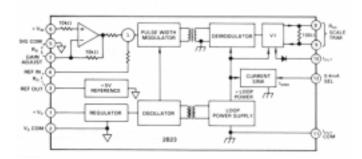
In data acquisition and control systems, the 2B23 may act as an isolated interface between the D/A converter output of a microcomputer analog I/O and standard 4 to 20mA or 0 to 20mA analog loops. In process control systems, the 2B23 may be used as a current output stage of a proportional controller to interface devices such as current-to-position converters and current-to-pneumatic transducers.
