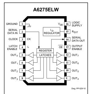
Note that the A6275EA (DIP) and the A6275ELW (SOIC) are electrically identical and share a common terminal number assignment.
