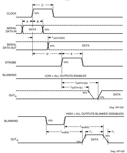
NOTE – Timing is representative of a 10 MHz clock. Higher speeds may be attainable; operation at high temperatures will reduce the specified maximum clock frequency.
