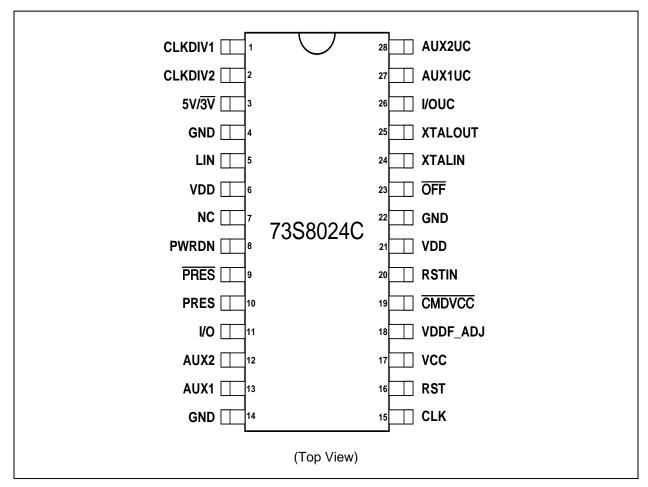
Figure 11: 73S8024C 28-SO Pin Out
