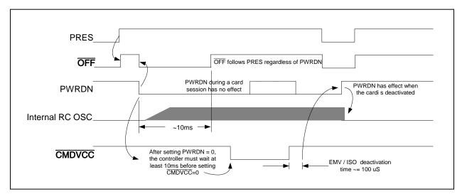
Figure 2: Power Down Mode Operation
