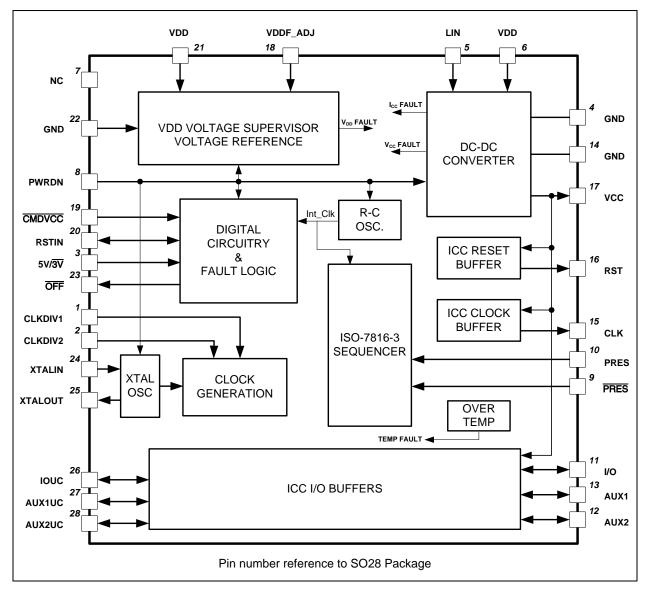
Figure 1: 73S8024C Block Diagram
