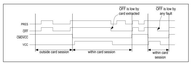
Figure 6: Timing Diagram – Management of the Interrupt Line OFF
