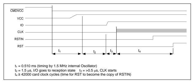
Figure 3: Activation Sequence – RSTIN low when CMDVCC goes low
