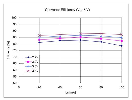
Figure 10: DC – DC Converter efficiency ( $V_{cc}$  = 5 V)
