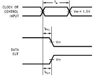
FIGURE 6. Propagation Delay, Pulse Width Waveforms
