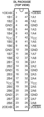
The dual-enable configuration gives the bus transceiver the capability to store data by simultaneous enabling of OEBA and OEAB. Each output reinforces its input in this transceiver configuration. Thus, when both control inputs are enabled and all other data sources to the two sets of bus lines are at high impedance, the bus lines will remain at their last states.
