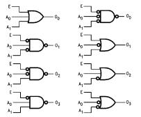
FIGURE 1. Gate Functions (Each Half)
