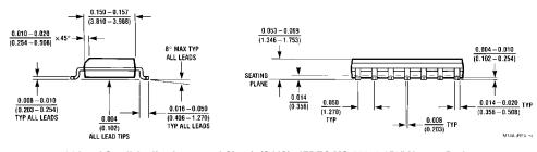
14-Lead Small Outline Integrated Circuit (SOIC), JEDEC MS-120, 0.150" Narrow Body Package Number M14A
