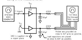
FIGURE 2. Simultaneous Switching Test Circuit
