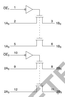
Figure 2. Logic Diagram
