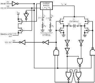
FIGURE 1. Logic Diagram for VCO
