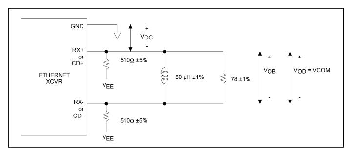
FIGURE 2: Test Load for CD± or RX±
