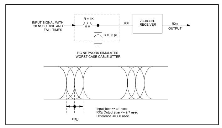
FIGURE 8: Receive Jitter Timing
