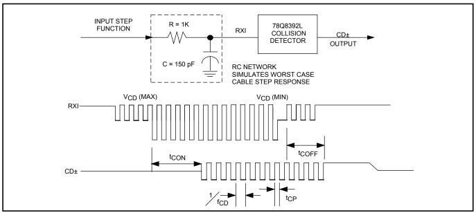
FIGURE 5: Collision Timing
