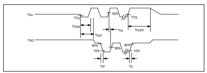
FIGURE 4: Transmitter Timing
