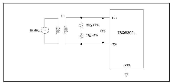
FIGURE 10: Test Circuit for TX± Input
