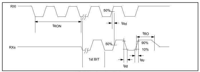
FIGURE 3: Receiver Timing
