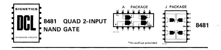
The 8481 is a Quad 2-Input NAND Gate with bare output collectors. Absence of an output pull-up structure allows the user complete freedom in the use of the 8481 in collector-logic (wired-AND) and similar applications. Proper pull-up resistor selection will allow as many as 30 outputs to be tied together.
