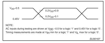
Figure 7. AC Testing Input/Output
