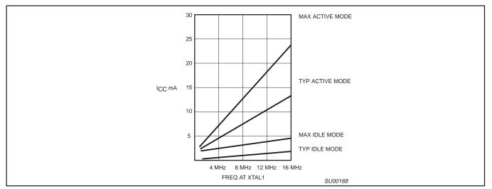
$\label{eq:Figure 9. I_CC} \textbf{Vs. FREQ.}$  Valid only within frequency specifications of the device under test
