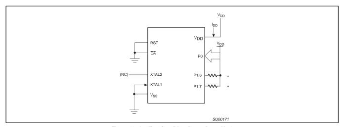
Figure 13.  $I_{DD}$  Test Condition, Power Down Mode All other pins are disconnected.  $V_{DD}$  = 2V to 5.5V
