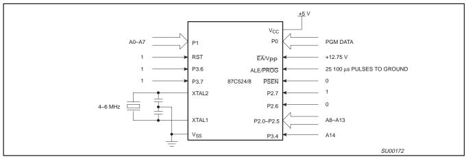
Figure 14. Programming Configuration
