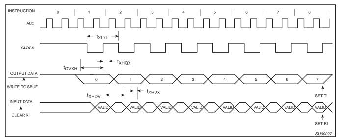
Figure 4. Shift Register Mode Timing
