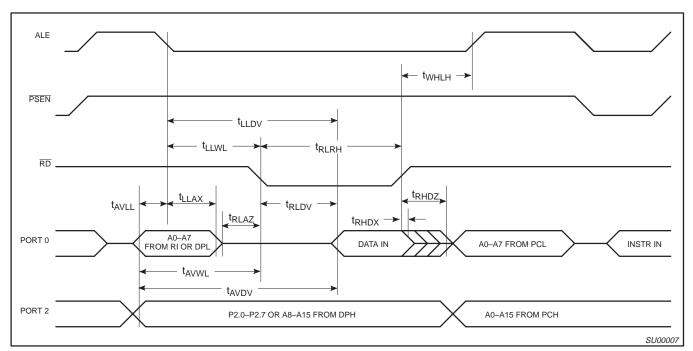
Figure 2. External Data Memory Read Cycle
