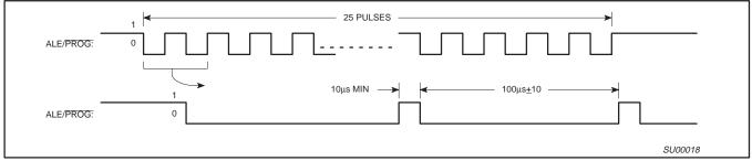
Figure 15. PROG Waveform
