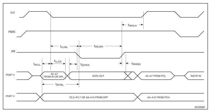
Figure 3. External Data Memory Write Cycle
