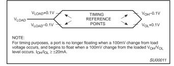
Figure 8. Float Waveform
