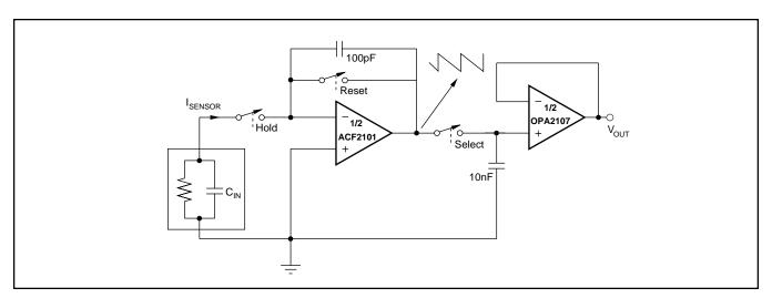
FIGURE 10. Programmable Current-to-Voltage Converter.
