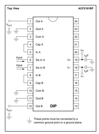
FIGURE 1b. Basic Circuit Connections, DIP.
