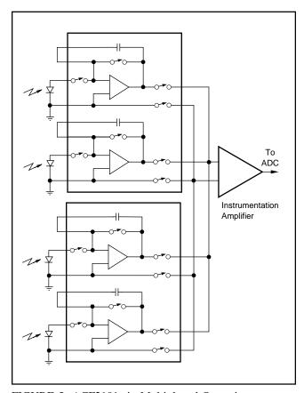
FIGURE 5. ACF2101s in Multiplexed Operation.
