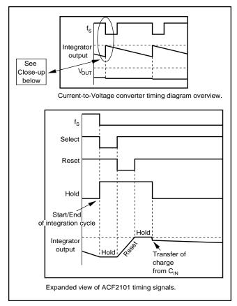
FIGURE 9. ACF2101 Current-to-Voltage Converter Timing Diagram.
