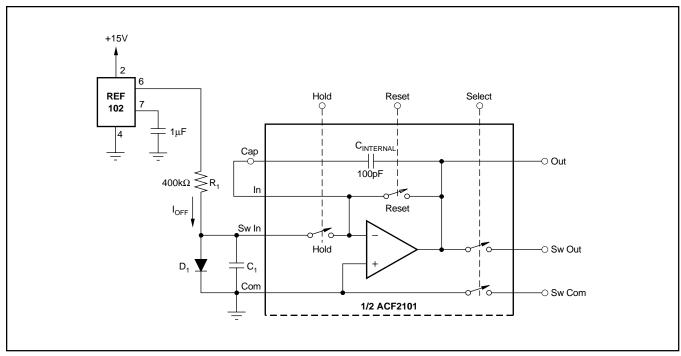
FIGURE 12. Using the ACF2101 with a Voltage Source.
