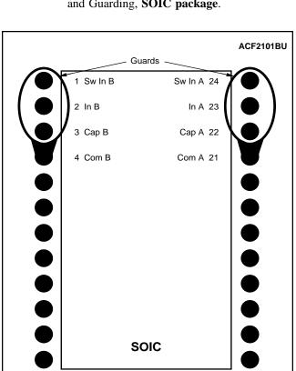
FIGURE 2a. PC Board Layout Showing "Guard" Traces for Input, **SOIC package**. Both top and bottom of board should be guarded.
