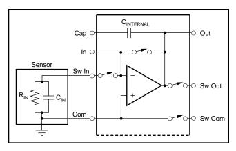
FIGURE 6. Capacitance of Circuit at Input of Integrator.
