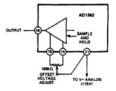
Figure 3. AD1362 Offset Voltage Adjustment
