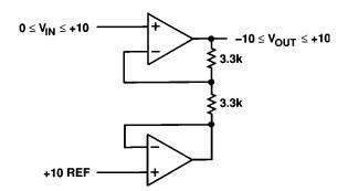
Figure 27. High Input Impedance Unipolar-to-Bipolar Conversion Circuit
