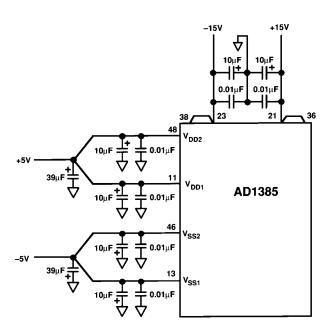
Figure 15. Recommended AD1385 Power Distribution. All  $10 \, \mu F$  and  $0.01 \, \mu F$  capacitors must have minimum lead length and be located as close as possible to the bypassed pins. Make all ground connections directly to the groundplane.
