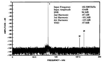
Figure 9. Full-Scale Sine Wave Power Spectral Density, ±10 V Range, 16384-Point FFT, 500 kHz Sample Rate
