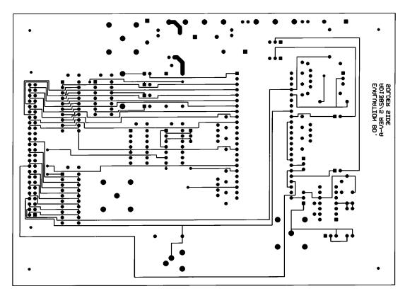
Figure 33. AD1385 Evaluation Board Layout, Layer 4 (Solder Side)
