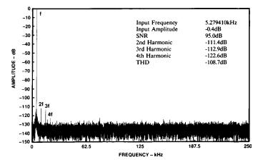
Figure 8. Full-Scale Sine Wave Power Spectral Density, ±10 V Range, 16384-Point FFT, 500 kHz Sample Rate
