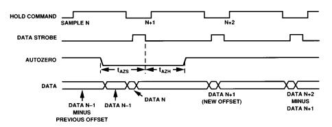
Figure 24. Autozero Cycle Operation
