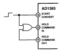
Figure 19. Connecting the AD1385 to Sample the Input Signal Asynchronously from the Clock
