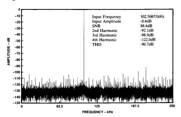
Figure 21. Full-Scale Power Spectral Density at  $T_{CASE}$  = +125°C, Calibration Performed at  $T_{CASE}$  = +25°C,  $\pm 5$  V Range, 16384-Point FFT, 500 kHz Sample Rate
