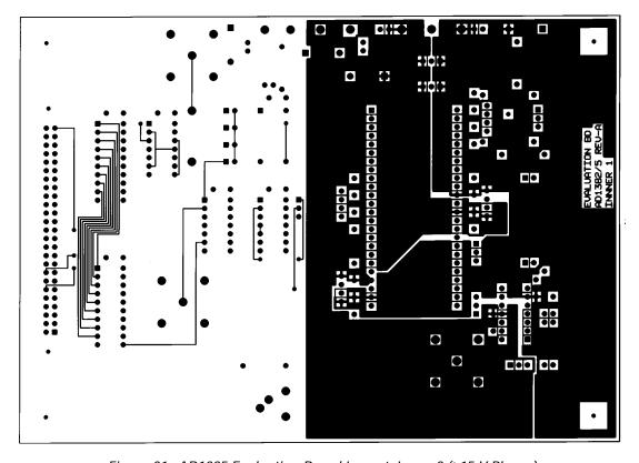
Figure 31. AD1385 Evaluation Board Layout, Layer 2 ( $\pm 15$  V Planes)
