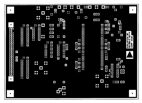
Figure 30. AD1385 Evaluation Board Layout, Layer 1 (Component Side)
