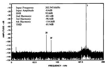
Figure 10. Full-Scale Sine Wave Power Spectral Density, ±10 V Range, 16384-Point FFT, 500 kHz Sample Rate
