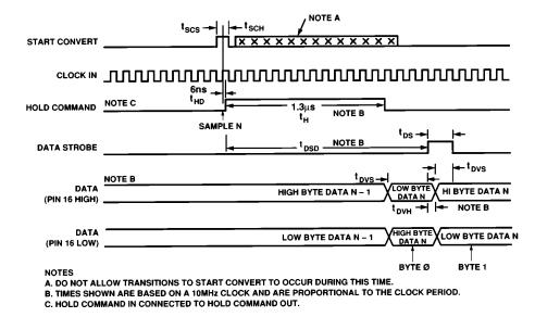
Figure 17. Start-Convert Controlled Conversion Timing
