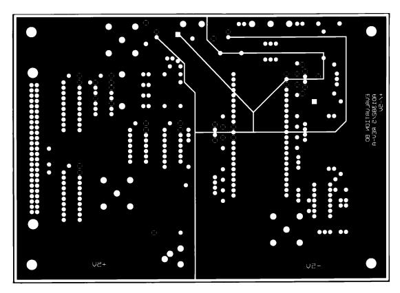
Figure 32. AD1385 Evaluation Board Layout, Layer 3 (±5 V Planes)
