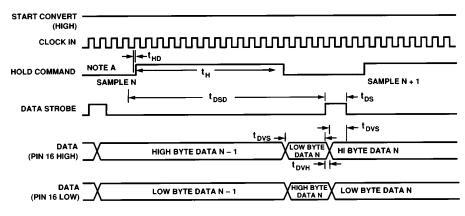
NOTE A: HOLD COMMAND IN CONNECTED TO HOLD COMMAND OUT
