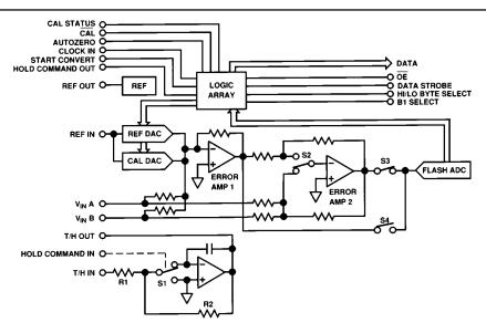
Figure 13. AD1385 Functional Block Diagram
