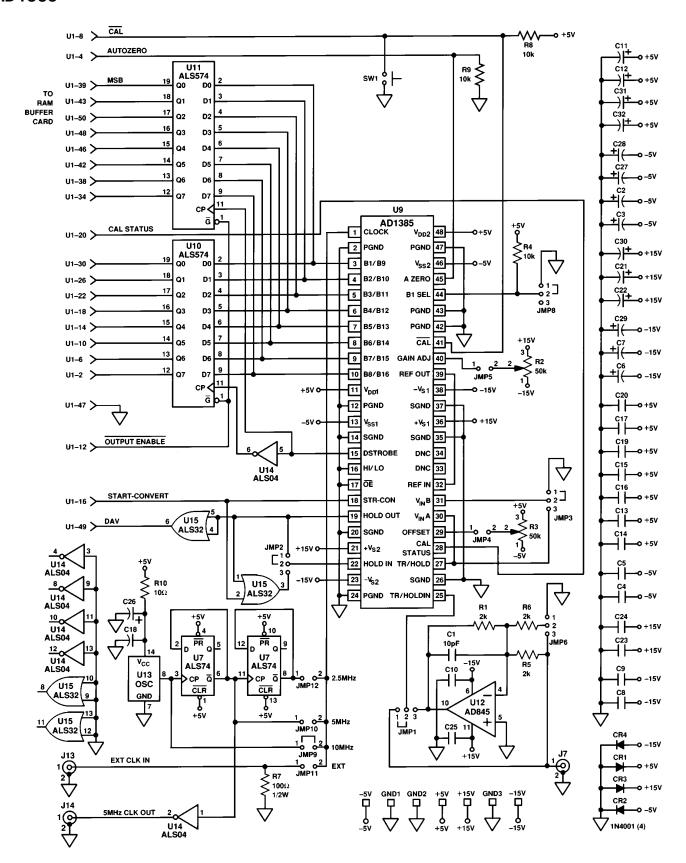
Figure 29. AD1385 Evaluation Board Schematic
