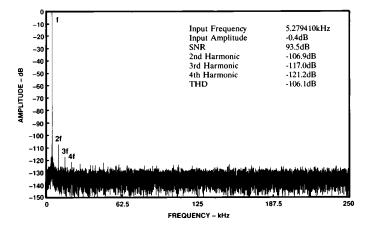
Figure 3. Full-Scale Sine Wave Power Spectral Density,  $\pm 5$  V Range, 16384-Point FFT, 500 kHz Sample Rate
