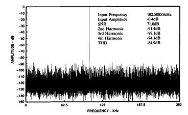
Figure 20. Full-Scale Power Spectral Density after Powerup at  $T_{CASE}$  = +25°C Without Calibration, ±5 V Range, 16384-Point FFT, 500 kHz Sample Rate. Compare with Figure 4.
