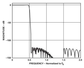
TPC 3. ADC Composite Filter Response (Pass-Band Section)
