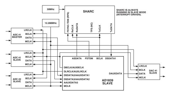
Figure 13. Aux Mode Connection to SHARC (Slave Mode)
