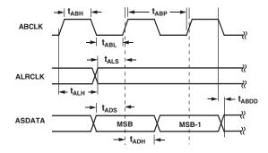
Figure 9. ADC Packed Mode Timing
