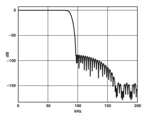
TPC 7. DAC Composite Filter Response,  $f_S = 192 \text{ kHz}$
