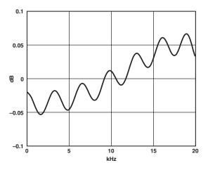
TPC 8. DAC Composite Filter Response,  $f_S = 48 \text{ kHz}$  (Pass-Band Section)
