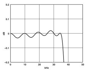
TPC 9. DAC Composite Filter Response,  $f_S = 96 \text{ kHz}$  (Pass-Band Section)
