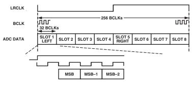
Figure 7. ADC Packed Mode 256
