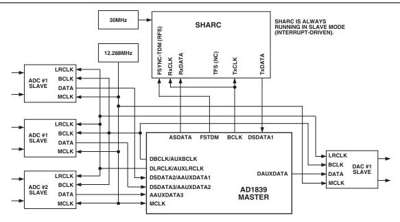
Figure 12. Aux Mode Connection to SHARC (Master Mode)
