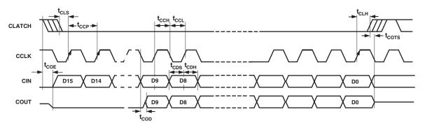
Figure 3. Format of SPI Timing
