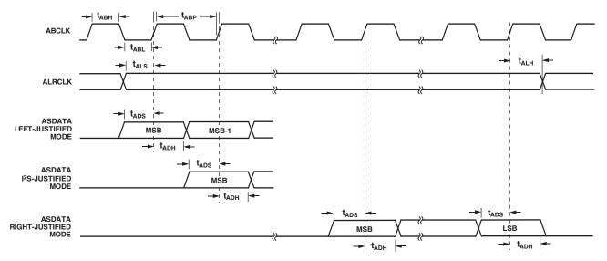
Figure 5. ADC Serial Mode Timing
