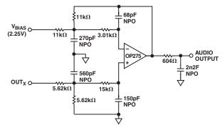
Figure 15. Typical DAC Output Filter Circuit
