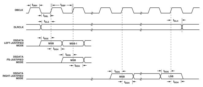
Figure 6. DAC Serial Mode Timing
