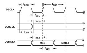
Figure 10. DAC Packed Mode Timing
