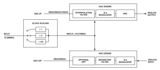
Figure 2. Modulator Clocking Scheme
