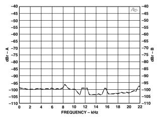
Figure 13. THD+N vs. Frequency at -0.5 dBFS
