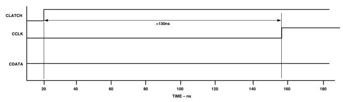
Figure 7. SPI Port Continuous CCLK Mode
