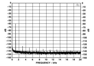
Figure 14. Dynamic Range: 1 kHz at -60 dB
