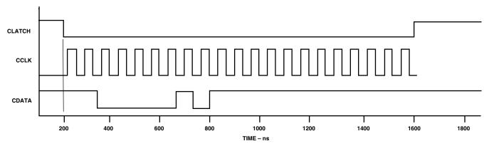
Figure 8. SPI Port Burst Mode
