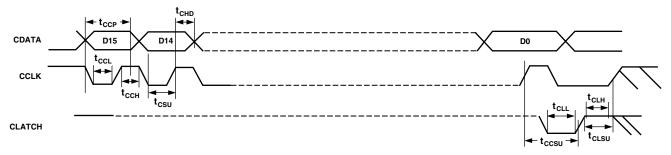
Figure 6. Serial Control Port Timing
