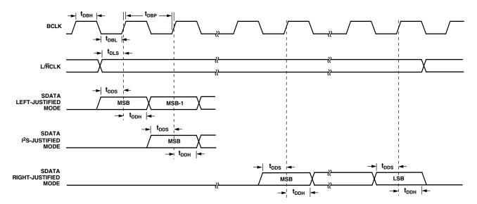
Figure 9. Serial Data Port Timing
