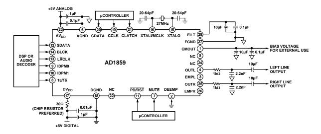
Figure 17. Recommended Circuit Connection (Without De-emphasis)
