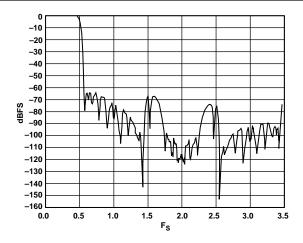
Figure 31. Digital Filter Signal Transfer Function to  $3.5 \times F_S$
