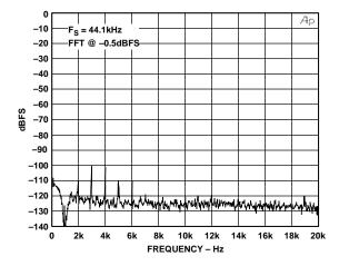
Figure 24. 1 kHz Tone at -0.5 dBFS (16K-Point FFT)
