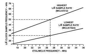
Figure 10. MCLK Frequency vs. L/R Clock Frequency
