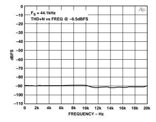
Figure 26. THD+N vs. Frequency at -0.5 dBFS
