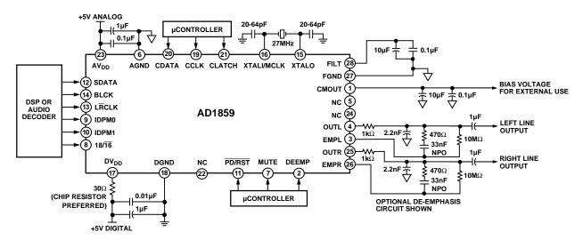
Figure 18. Recommended Circuit Connection (With De-emphasis)
