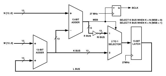
Figure 33. Numerically Controlled Oscillator Circuit
