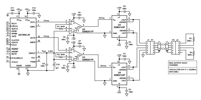
Figure 32. 600 Ohm Balanced Line Driver
