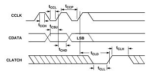
Figure 22. Serial Control Port Timing
