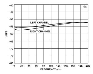
Figure 28. Power Supply Rejection to 300 mV p-p on AV<sub>DD</sub>
