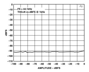
Figure 27. THD+N vs. Amplitude at 1 kHz
