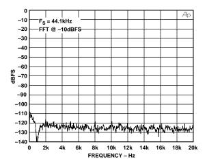
Figure 25. 1 kHz Tone at -10 dBFS (16K-Point FFT)
