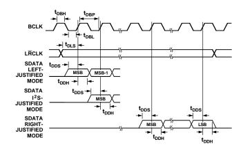
Figure 20. Serial Data Port Timing
