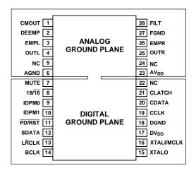
Figure 19. Recommended Ground Plane
