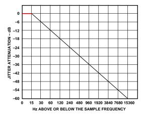
Figure 1. Digital PLL Jitter Rejection
