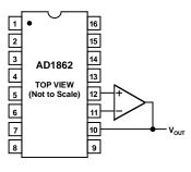
Figure 9. External Amplifier Connections
