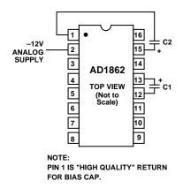
Figure 8. Noise Reduction Capacitors
