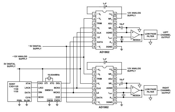
Figure 13. High Performance 20-Bit 8 × Oversampling CD Player Application
