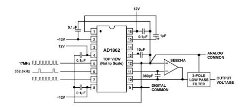
Figure 10. Recommended Test Circuit
