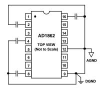
Figure 7. Grounding and Bypassing Recommendations
