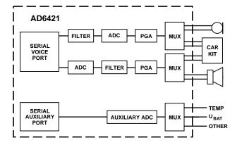
Figure 3. Audio/Auxiliary Section of the AD6421
