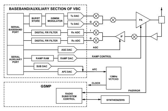
Figure 2. Control of Radio Subsystem
