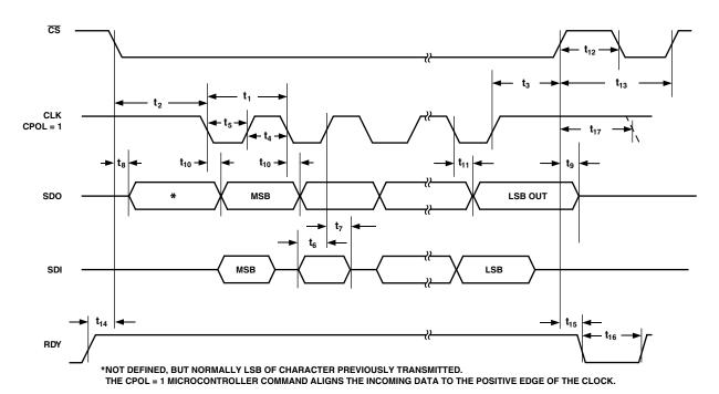
Figure 2a. CPHA = 1 Timing Diagram
