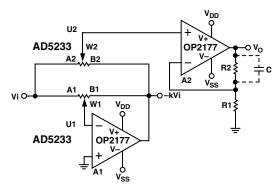
Figure 16. Bipolar Programmable Gain Amplifier
