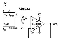
Figure 15. Programmable Voltage Reference
