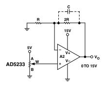
Figure 14. 15 V Voltage Span Control
