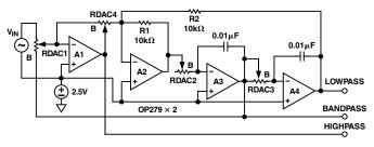
Figure 18. Programmable Stable Variable Filter
