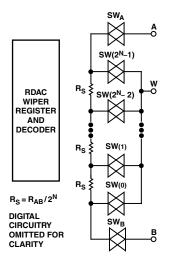
Figure 9. Equivalent RDAC Structure (Patent Pending)
