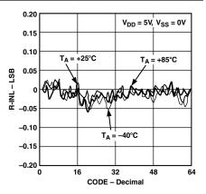
TPC 3. R-INL vs. Code,  $T_A = -40$ °C, +25°C, +85°C Overlay,  $R_{AB} = 10 \text{ k}\Omega$
