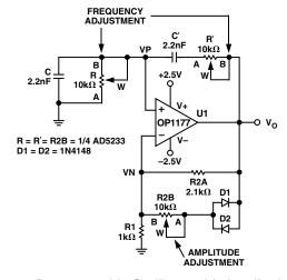
Figure 21. Programmable Oscillator with Amplitude Control
