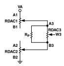
Figure 29. Doubling AD5233 from 6-Bit to 12-Bit
