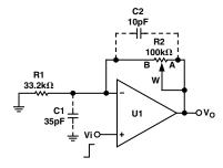
Figure 13. Typical Noninverting Gain Amplifier
