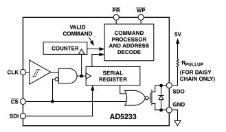
Figure 3. Equivalent Digital Input-Output Logic
