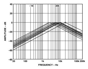
Figure 19. Programmed Center Frequency Bandpass Response
