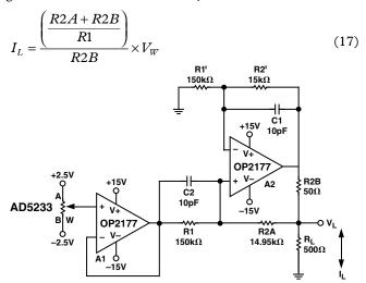
Figure 25. Programmable Bidirectional Current Source
