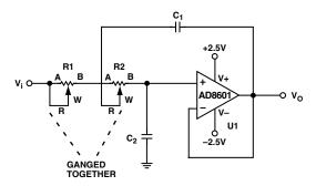
Figure 17. Sallen Key Low-Pass Filter
