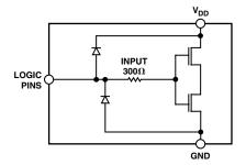
Figure 4a. Equivalent ESD Digital Input Protection
