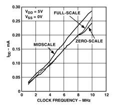
TPC 9.  $I_{DD}$  vs. Clock Frequency,  $R_{AB}=10~k\Omega$
