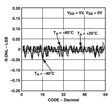
TPC 4. R-DNL vs. Code,  $T_A = -40$ °C, +25°C, +85°C Overlay,  $R_{AB} = 10$  k $\Omega$
