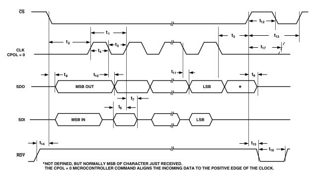
Figure 2b. CPHA = 0 Timing Diagram
