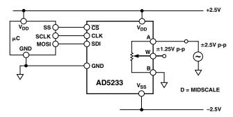
Figure 12. Bipolar Operation from Dual Supplies
