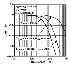
TPC 10. -3 dB Bandwidth vs. Resistance. Test Circuit 7.
