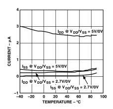
TPC 8.  $I_{DD}$  vs. Temperature,  $R_{AB}=10~k\Omega$
