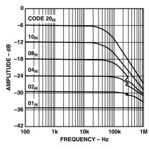
TPC 14. Gain vs. Frequency vs. Code,  $R_{AB} = 100 \text{ k}\Omega$ . Test Circuit 7.
