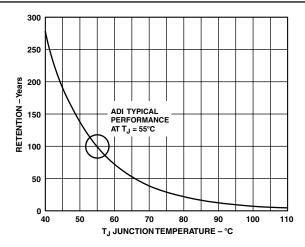
Figure 11. Flash/EE Memory Data Retention
