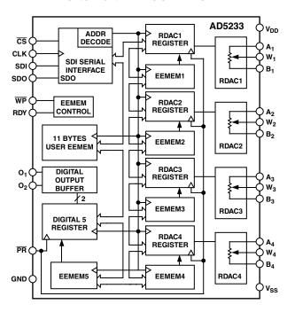
The linear step increment and decrement commands allows the setting in the RDAC register to be moved UP or DOWN, one step at a time. For logarithmic changes in wiper setting, a left/right bit shift command adjusts the level in  $\pm 6$  dB steps.
