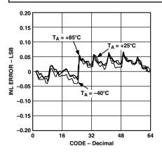
TPC 1. INL vs. Code,  $T_A = -40$ °C, +25°C, +85°C Overlay,  $R_{AB} = 10 \text{ k}\Omega$
