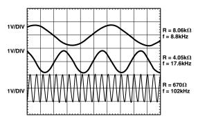
Figure 22. Programmable Oscillation
