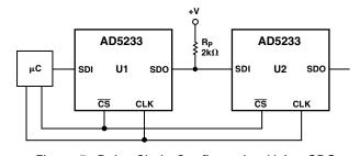
Figure 5. Daisy Chain Configuration Using SDO
