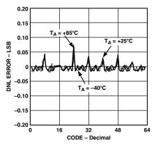
TPC 2. DNL vs. Code,  $T_A = -40$ °C, +25°C, +85°C Overlay,  $R_{AB} = 10 \text{ k}\Omega$
