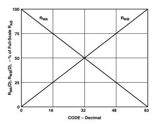
Figure 1.  $R_{WA}(D)$  and  $R_{WB}(D)$  vs. Decimal Code
