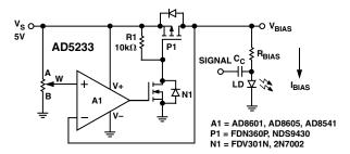
Figure 23. Programmable Booster Voltage Source
