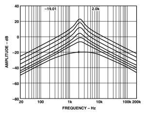
Figure 20. Programmed Amplitude Bandpass Response
