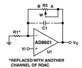
Figure 30. Linear Gain Control with Tracking Resistance Tolerance, and Temperature Coefficient
