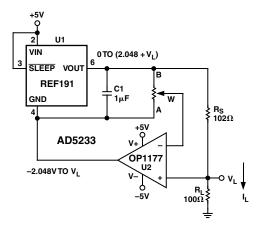
Figure 24. Programmable 4-to-20 mA Current Source
