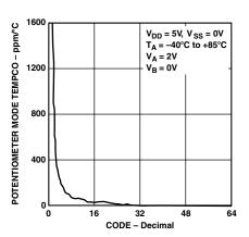
TPC 6.  $\Delta V_{WB}/\Delta T$  vs. Code,  $R_{AB}=10~k\Omega$
