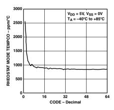
TPC 5.  $\Delta R_{WB}/\Delta T$  vs. Code,  $R_{AB}=$  10  $k\Omega$
