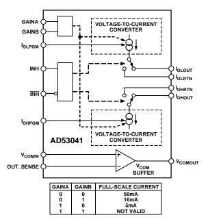
The AD53041 is available in a 20-lead, PSOP package with a built-in-heatsink and is specified to operate over the ambient commercial temperature range from  $-25^{\circ}$ C to  $+85^{\circ}$ C.
