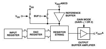
Figure 4. Single DAC Channel Architecture
