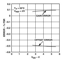
TPC 10. Offset Error and Gain Error vs. V<sub>DD</sub>
