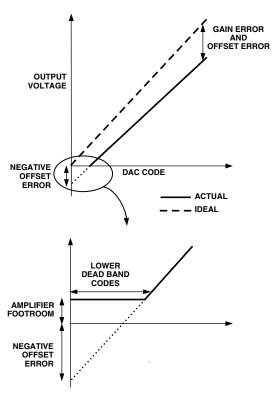
Figure 2. Transfer Function with Negative Offset  $(V_{REF} = V_{DD})$
