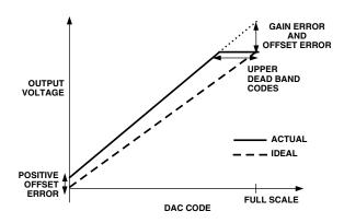
Figure 3. Transfer Function with Positive Offset
