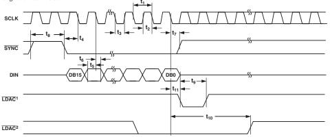
Figure 1. Serial Interface Timing Diagram
