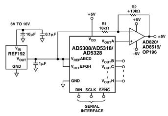
Figure 16. Bipolar Operation with the AD5308/AD5318/AD5328
