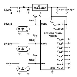
Figure 17. AD5308/AD5318/AD5328 in an Opto-Isolated Interface
