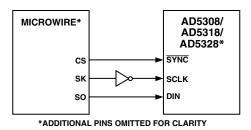
Figure 14. MICROWIRE to AD5308/AD5318/ AD5328 Interface
