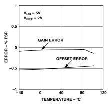
TPC 9. AD5308 Offset Error and Gain Error vs. Temperature
