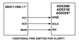
Figure 12. 68HC11/68L11 to AD5308/AD5318/ AD5328 Interface
