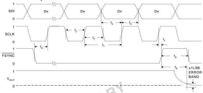
Figure 1B. Detail Timing Diagram
