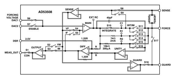
Figure 3. Guarded Current Force/Voltage Measure, I<sub>RANGE 1</sub>: I ≤ 2 mA
