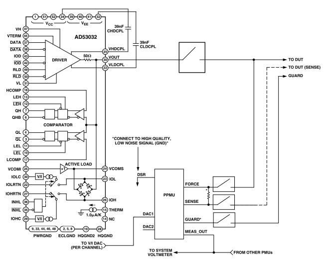
Figure 4. Recommended Use of the PPMU with a DCL
