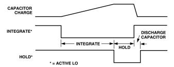
Figure 1. Integrate/Current Measure Timing Diagram
