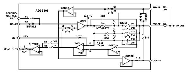
Figure 2. Guarded Voltage Force/Current Measure, I<sub>RANGE 1</sub>: I ≤ 2 mA
