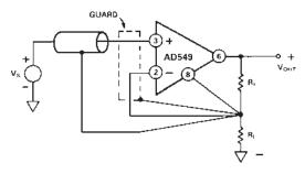
Figure 5. Noninverting Amplifier with Guard
