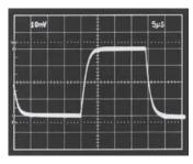
Figure 11. Inverter Pulse Response with 1  $M\Omega$  Source and Feedback Resistance, 1 pF Feedback Capacitance
