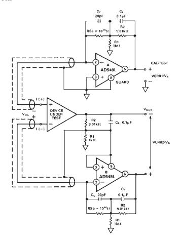
Figure 16. Sample and Difference Circuit for Measuring Electrometer Leakage Currents
