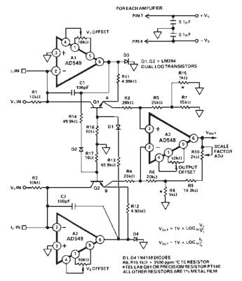
Figure 21. Log Ratio Amplifier
