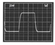
Figure 9. Follower Pulse Response from 1  $M\Omega$ Source Resistance, Case Bootstrapped
