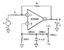
Figure 7. Alternate Offset Null Circuit for Inverter
