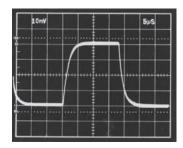
Figure 8. Follower Pulse Response from 1  $M\Omega$ Source Resistance, Case Not Bootstrapped
