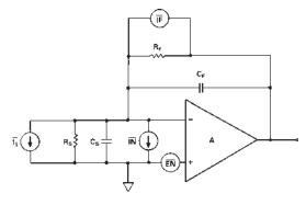
Figure 19. Photodiode Preamp Noise Sources
