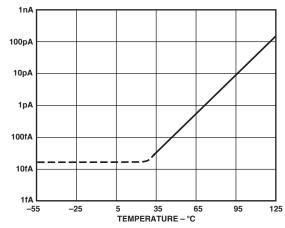
Figure 1. Input Bias Current vs. Ambient Temperature
