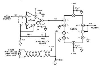
Figure 22. Temperature Compensated pH Probe Amplifier
