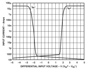
Figure 12. Input Current vs. Differential Input Voltage
