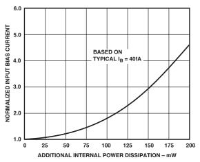
Figure 2. Input Bias Current vs. Additional Power Dissipation
