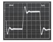
Figure 10. Inverter Pulse Response with 1  $M\Omega$  Source and Feedback Resistance
