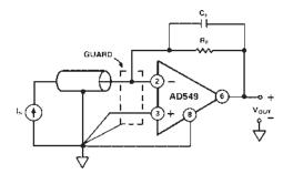
Figure 4. Inverting Amplifier with Guard
