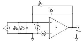
Figure 18. Photodiode Preamp DC Error Sources
