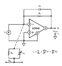
Figure 3. Sources of Parasitic Leakage Currents
