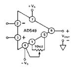
Figure 6. Standard Offset Null Circuit
