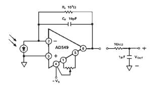
Figure 17. Photodiode Preamp
