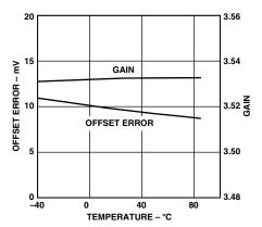
Figure 7. Offset Error and Gain vs. Temperature
