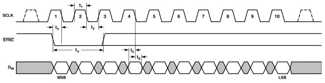
Figure 3. 10-Bit Write (SHA Mode and Both Readback Modes)
