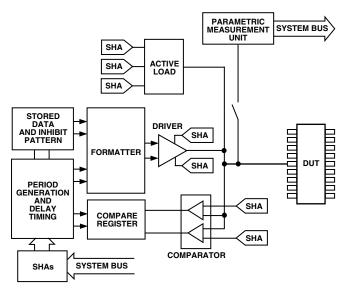
Figure 18. AD5533 in an ATE System
