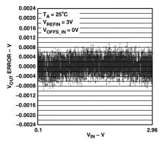
Figure 6.  $V_{IN}$  to  $V_{OUT}$  Accuracy after Offset and Gain Adjustment
