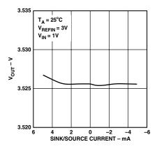
Figure 8. V<sub>OUT</sub> Source and Sink Capability
