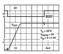
Figure 9. Acquisition Time and Output Settling Time
