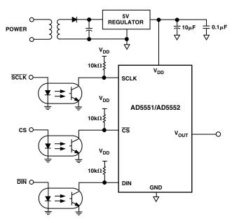
Figure 9. AD5551/AD5552 in an Optocoupler Interface
