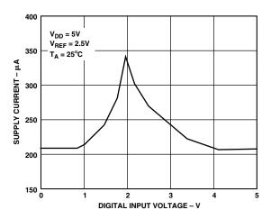
TPC 9. Supply Current vs. Digital Input Voltage
