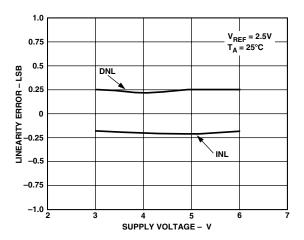
TPC 3. Linearity Error vs. Supply Voltage
