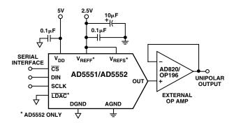
Figure 3. Unipolar Output
