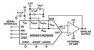
Figure 4. Bipolar Output (AD5552 Only)
