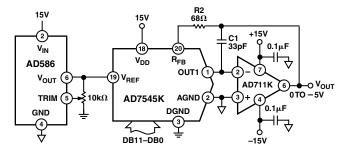
Figure 11. Low-Power 12-Bit CMOS DAC Application
