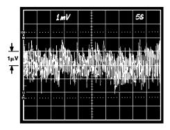
Figure 3. 0.1 Hz to 10 Hz Noise
