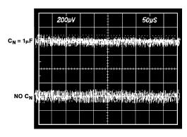
Figure 4. Effect of 1 μF Noise Reduction Capacitor on Broadband Noise
