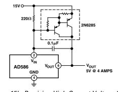
Figure 15b. Precision High-Current Voltage Source
