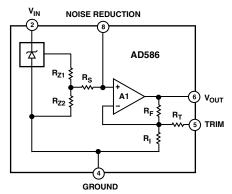
NOTE: PINS 1, 3, AND 7 ARE INTERNAL TEST POINTS. MAKE NO CONNECTIONS TO THESE POINTS.
