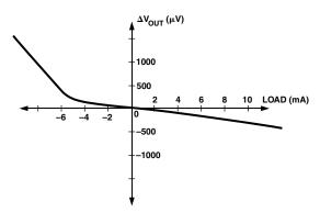
Figure 8. Typical Load Regulation Characteristics
