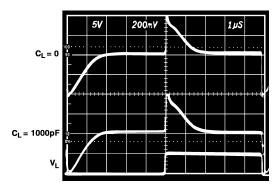
Figure 7b. Output Response with Capacitive Load
