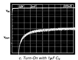
Figure 5. Turn-On Characteristics
