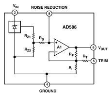
NOTE: PINS 1, 3, AND 7 ARE INTERNAL TEST POINTS.
