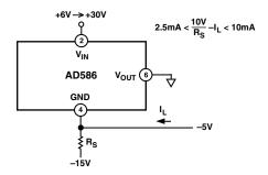
Figure 10. AD586 as a Negative 5 V Reference
