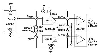
Figure 12. AD586 as a 5 V Reference for a CMOS Dual DAC
