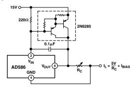
Figure 15a. Precision High-Current Current Source
