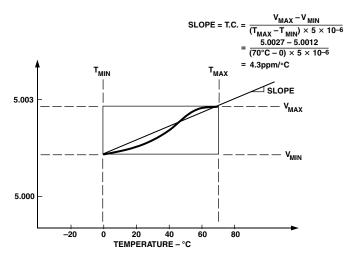
Figure 9. Typical AD586L Temperature Drift
