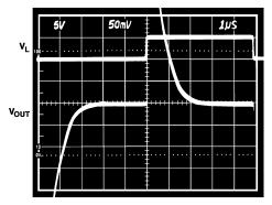
Figure 6b. Large-Scale Transient Response
