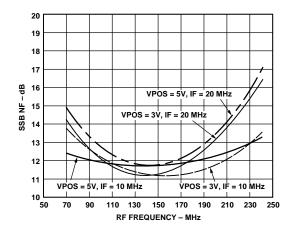
Figure 13. Mixer Noise Figure vs. Frequency
