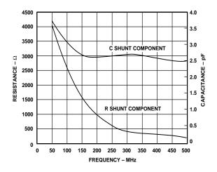
Figure 14. Mixer Input Impedance vs. Frequency, VPOS = 3 V, V GAIN = 0.8 V
