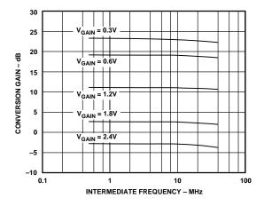
Figure 16. Mixer Conversion Gain vs. IF, T = +25°C, VPOS = 3 V, VREF = 1.5 V
