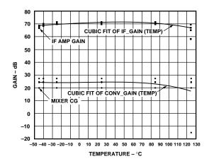
Figure 17. Mixer Conversion Gain and IF Amplifier Gain vs. Temperature, VPOS = 3 V, VGAIN = 0.3 V, VREF = 1.5 V, VREF
