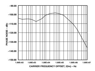
Figure 22. PLL Phase Noise L (F) vs. Frequency, VPOS = 3 V, C3 =  $0.1 \,\mu\text{F}$ , IF =  $10.7 \,\text{MHz}$
