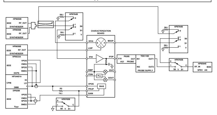
Figure 1. Mixer/Amplifier Test Set
