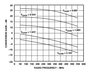
Figure 15. Mixer Conversion Gain vs. Frequency,  $T = +25^{\circ}\text{C}$ , VPOS = 2.7 V, VREF = 1.35 V, IF = 10.7 MHz
