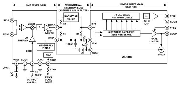
Figure 21. Applications Diagram for Common IFs and Filter Impedances
