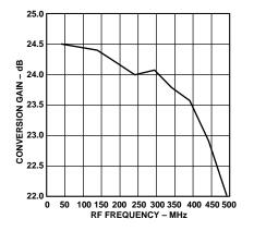
Figure 3. Mixer Conversion Gain vs. Frequency
