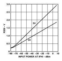
Figure 5. IF RSSI Output vs. Supply Voltage (Ambient Temperature)
