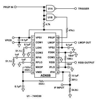
Figure 1. IF Test Board Schematic
