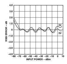
Figure 8. RSSI Error vs. Input Power
