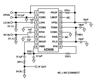
Figure 2. Mixer Test Board Schematic
