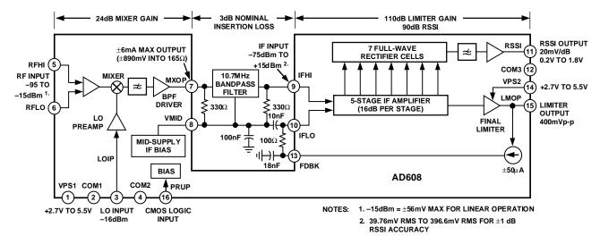
Figure 20. Functional Block Diagram
