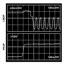
Figure 15. Limiter Power-Up Response Time
