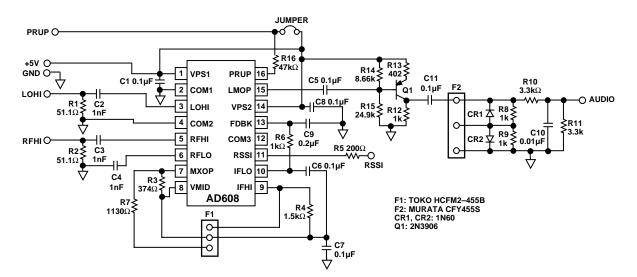
Figure 23. Narrowband FM Application at 450 kHz or 455 kHz
