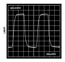
Figure 13. Limiter Rise and Fall Times
