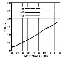
Figure 6. IF RSSI Output vs. Temperature (3 V Supply)
