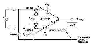
*Figure 18c. Ground Returns for Bias Currents with AC Coupled Inputs*
