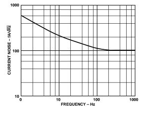
Figure 5. Current Noise Spectral Density vs. Frequency
