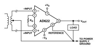
Figure 18a. Ground Returns for Bias Currents with Transformer Coupled Inputs
