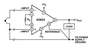
Figure 18b. Ground Returns for Bias Currents with Thermocouple Inputs
