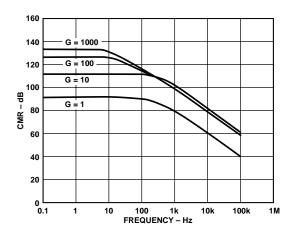
Figure 6. CMR vs. Frequency, RTI, Zero to 1  $k\!\Omega$  Source Imbalance
