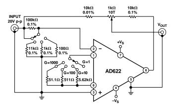
Figure 13. Settling Time Test Circuit
