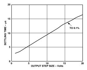
Figure 10. Settling Time vs. Step Size (G = 1)
