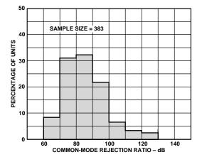
Figure 2. Typical Distribution of Common-Mode Rejection
