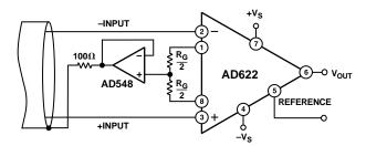
Figure 16. Common-Mode Shield Driver
