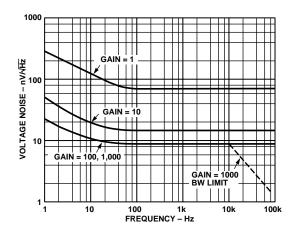
Figure 4. Voltage Noise Spectral Density vs. Frequency, (G = 1-1000)
