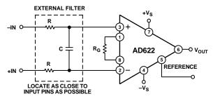
Figure 15. Circuit to Attenuate RF Interference
