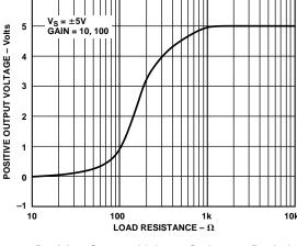
Figure 4. Positive Output Voltage Swing vs. Resistive Load
