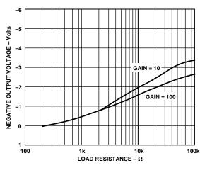
Figure 5. Negative Output Voltage Swing vs. Resistive Load
