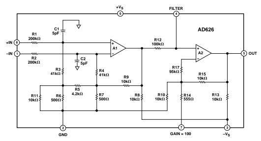
Figure 28. Simplified Schematic
