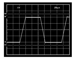
Figure 19. Large Signal Pulse Response.  $V_S = \pm 5 \ V$ , G = 10
