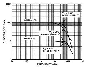
Figure 7. Closed-Loop Gain vs. Frequency
