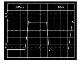
Figure 21. Large Signal Pulse Response.  $V_S = +5 V$ , G = 10
