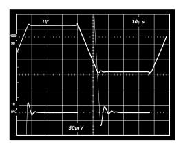
Figure 25. Settling Time.  $V_S = +5 V$ , G = 10
