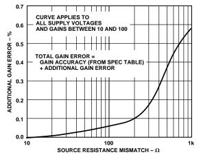
Figure 12. Additional Gain Error vs. Source Resistance Mismatch
