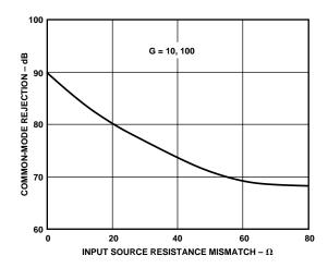
Figure 11. Common-Mode Rejection vs. Input Source Resistance Mismatch
