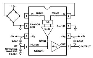
Figure 34. A Typical Bridge Application
