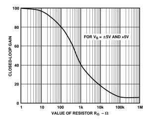
Figure 17. Closed-Loop Gain vs. R<sub>G</sub>
