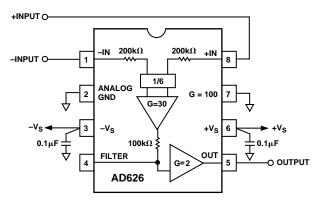
Figure 30. AD626 Configured for a Gain of 100
