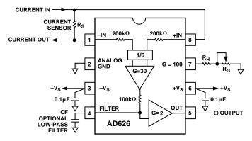
Figure 33. Current Sensor Interface
