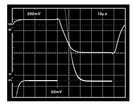
Figure 26. Settling Time.  $V_S = +5 \text{ V}$ , G = 100
