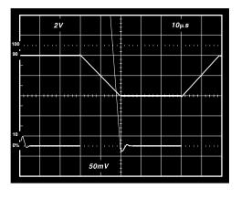
Figure 23. Settling Time.  $V_S = \pm 5 V$ , G = 10
