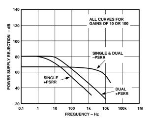
Figure 18. Power Supply Rejection vs. Frequency
