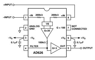
Figure 29. AD626 Configured for a Gain of 10
