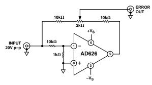
Figure 27. Settling Time Test Circuit
