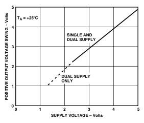
Figure 2. Positive Output Voltage Swing vs. Supply Voltage
