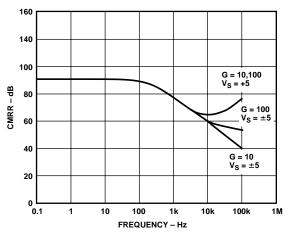
Figure 8. Common-Mode Rejection vs. Frequency
