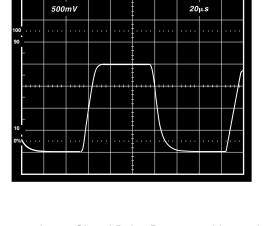
Figure 22. Large Signal Pulse Response.  $V_S = +5 V$ , G = 100
