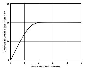
Figure 6. Change in Input Offset Voltage vs. Warm-Up
