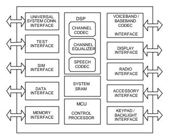
FIGURE 1. AD6528 FUNCTIONAL BLOCK DIAGRAM
