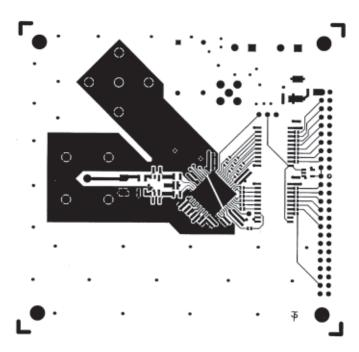
Figure 15. AD6644ST/PCB Top Side Copper
