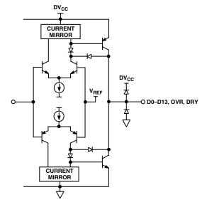
Figure 5. Digital Output Stage
