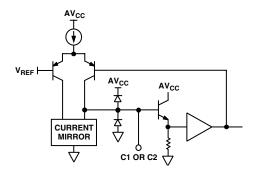
Figure 4. Compensation Pin, C1 or C2
