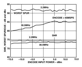
TPC 15. SNR, Worst Spurious vs. Clamped Encode Power (See Figure 8)
