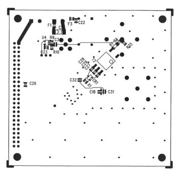
Figure 16. AD6644ST/PCB Bottom Side Silkscreen
