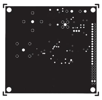
Figure 18. AD6644ST/PCB Ground Layer – Layers 2 and 5 (Negative)
