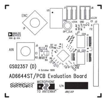
Figure 14. AD6644ST/PCB Top Side Silkscreen
