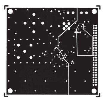
Figure 19. AD6644ST/PCB "Split" Power Layer – Layers 3 and 4 (Negative)
