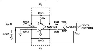
Figure 11. DC-Coupled Analog Input Circuit
