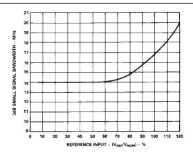
Figure 18. Small Signal Bandwidth vs. DC Reference Level
