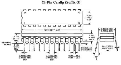
1. LEAD NO. 1 IDENTIFIED BY DOT OR NOTCH. 2. CERDIP LEADS WILL BE EITHER TIN PLATED OR SOLDER DIPPED IN ACCORDANCE WITH MIL-M-38510 REQUIREMENTS.
