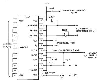
Figure 7. 5 V REFIN/1 V Unbuffered Unipolar Output
