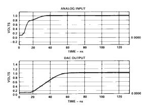
Figure 25. Typical Analog Settling Characteristic
