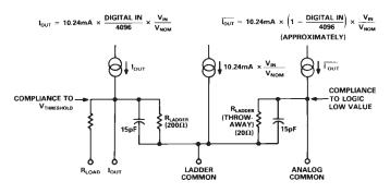
Figure 4. Equivalent Output Circuit
