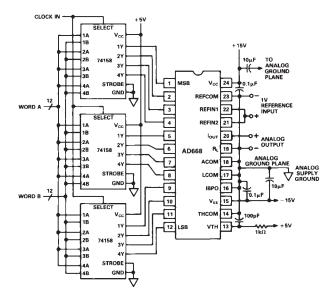
Figure 23. Settling Time Circuit
