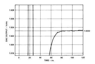
Figure 22. Typical Digital Settling Characteristics
