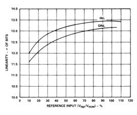
Figure 16. Linearity vs. Reference Level
