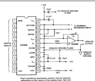
Figure 10. 1 V REFIN/-10 V Unipolar Buffered Output
