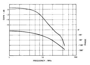
Figure 17. Large Signal Gain and Phase Response
