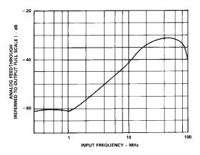
Figure 20. Analog Feedthrough vs. Frequency
