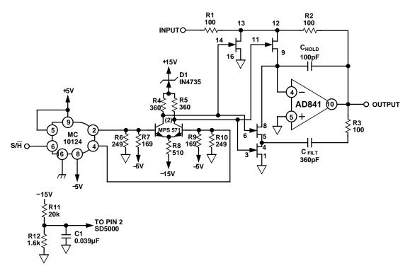
Figure 27. High Performance, Low Cost Deglitching Circuit
