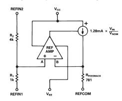
Figure 5. Equivalent Analog Input Circuitry
