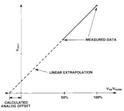
Figure 1. Derivation of Analog Offset Voltage
