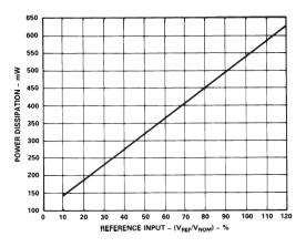
Figure 15. Power Consumption vs. Reference Level
