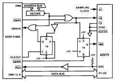
Figure 12. AD679 to ADSP-2100A Interface
