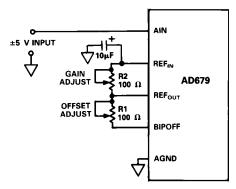
Figure 5. Bipolar Input Connections with Gain and Offset Trims
