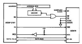
Figure 11. AD679 to ADSP-2101 Interface
