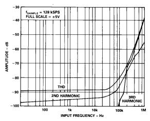
Figure 13. Harmonic Distortion vs. Input Frequency (–0.5 dB Input)
