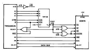
Figure 9. AD679 to TMS320C25 Interface
