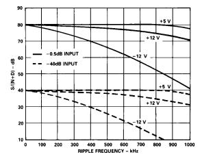
Figure 18. Power Supply Rejection ( $f_{IN} = 10 \text{ kHz}$ ,  $f_{SAMPLE} = 128 \text{ kSPS}$ ,  $V_{RIPPLE} = 0.1 \text{ V p-p}$ )
