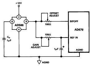
Figure 7. Bipolar Input with Gain and Offset Trims
