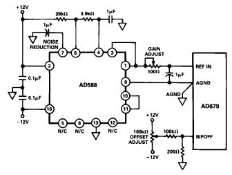
Figure 8. Unipolar Input with Gain and Offset Trims
