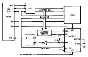
Figure 10. AD679 to 80186 DMA Interface
