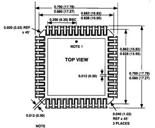
1. PIN 1 INDICATOR IS ON THE BOTTOM OF THE PACKAGE.
