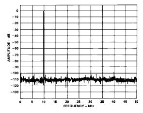
Figure 16. 5-Plot Averaged 2048 Point FFT at 128 kSPS,  $f_{\rm IN}$  = 10.009 kHz
