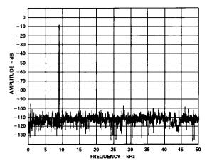
Figure 17. Nonaveraged IMD Plot for  $f_{\rm IN}$  = 9.08 kHz ( $f_a$ ), 9.58 kHz ( $f_b$ ) at 128 kSPS
