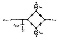
Figure 4. Load Circuit for Bus Timing Specifications
