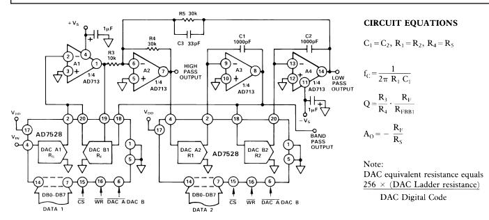
Figure 18. A Programmable State Variable Filter Circuit
