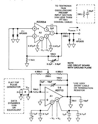
Figure 1. Settling Time Test Circuit
