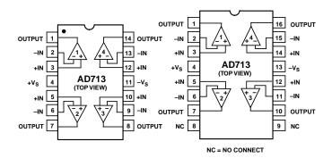
The AD713 is offered in a 16-pin SOIC, 14-pin plastic DIP and hermetic cerdip package.
