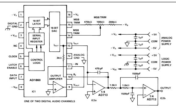
Figure 9. A D/A Converter Circuit for Digital Audio
