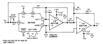
Figure 17. Bipolar Operation
