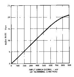
TPC 18. Slew Rate vs. Input Error Signal
