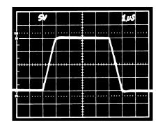
Figure 15. Transient Response,  $R_1 = 2 k\Omega$ ,  $C_1 = 500 pF$
