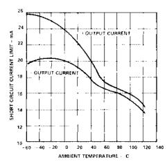
TPC 8. Short-Circuit Current Limit vs. Temperature
