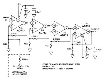
Figure 7. A High Speed Four Op Amp Cascaded Amplifier Circuit
