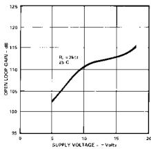
TPC 11. Open-Loop Gain vs. Supply Voltage
