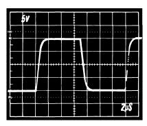
Figure 6. The Pulse Response of the High Speed Instrumentation Amplifier. Gain = 10
