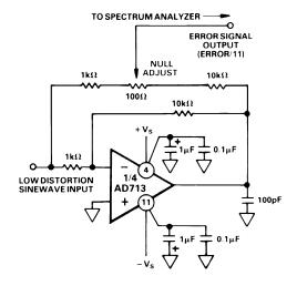
Figure 8. THD Test Circuit
