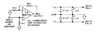
\*THE SIGNAL INPUT (1kHz SINFWAVF, 2V p-p) IS APPLIED TO ONE AMPLIFIER AT A TIME. THE OUTPUTS OF THE OTHER THREE AMPLIFIERS ARE THEN MEASURED FOR CROSSTALK.
