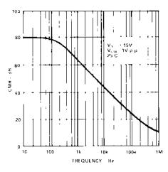
TPC 13. Common Mode Rejection vs. Frequency
