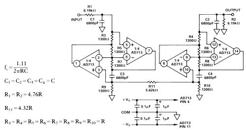
Figure 19. A 1/3 Octave Filter Circuit
