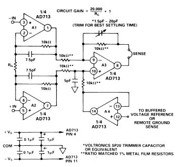
Figure 5. A High Speed Instrumentation Amplifier Circuit Table I provides a performance summary for this circuit. The photo of Figure 6 shows the pulse response of this circuit for a gain of 10.
