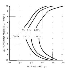
TPC 15. Output Swing and Error vs. Settling Time
