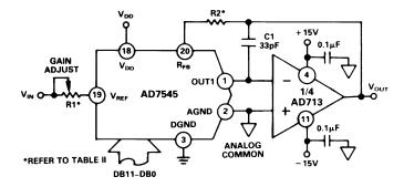
Figure 16. Unipolar Binary Operation
