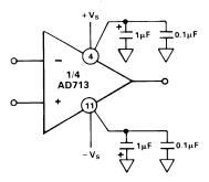
Figure 4. Recommended Power Supply Bypassing
