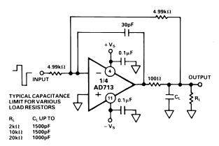
Figure 14. Circuit for Driving a Large Capacitance Load
