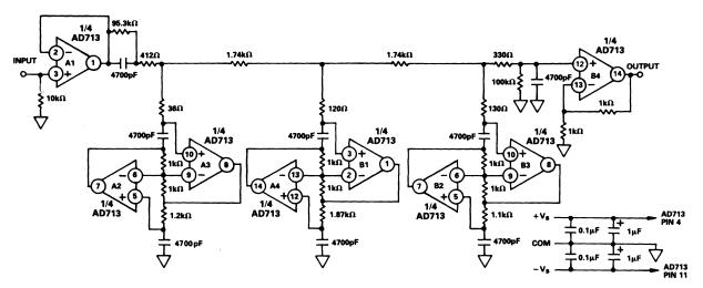
Figure 21. An Antialiasing Filter
