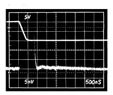
Figure 3. Settling Characteristics to –10 V Step. Upper Trace: Output of AD713 Under Test (5 V/div). Lower Trace: Amplified Error Voltage (0.01%/ div)
