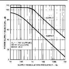
TPC 12. Power Supply Rejection vs. Frequency
