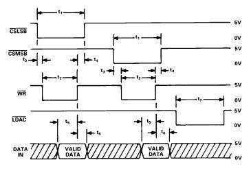
Figure 7. AD7248A Write Cycle Timing Diagram
