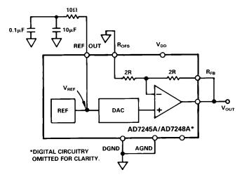
Figure 8. Unipolar (0 to +10 V) Configuration
