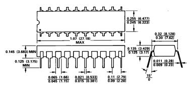
LEAD NO. 1 IDENTIFIED BY DOT OR NOTCH LEADS ARE SOLDER OR TIN-PLATED KOVAR OR ALLOY 42
