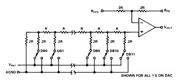
Figure 1. D/A Simplified Circuit Diagram
