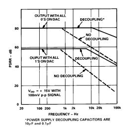
Power Supply Rejection Ration vs. Frequency
