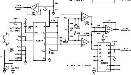
Figure 11. Programmable Function Generator
