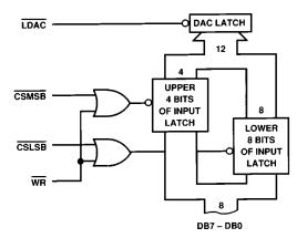
Figure 6. AD7248A Input Control Logic
