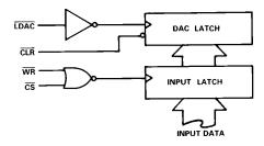
Figure 4. AD7245A Input Control Logic
