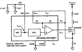
Figure 10. Programmable Current Sink
