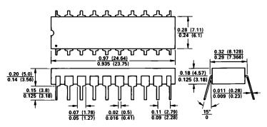
LEAD NO. 1 IDENTIFIED BY DOT OR NOTCH LEADS ARE SOLDER OR TIN-PLATED KOVAR OR ALLOY 42
